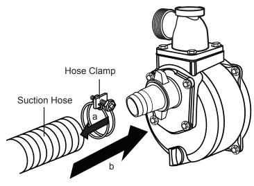
4. Slide a Hose Clamp over the other end of the suction hose (a). Slide the Intake Strainer into the end of the suction hose (b). Use a screwdriver to tighten the Hose Clamp until secure.
